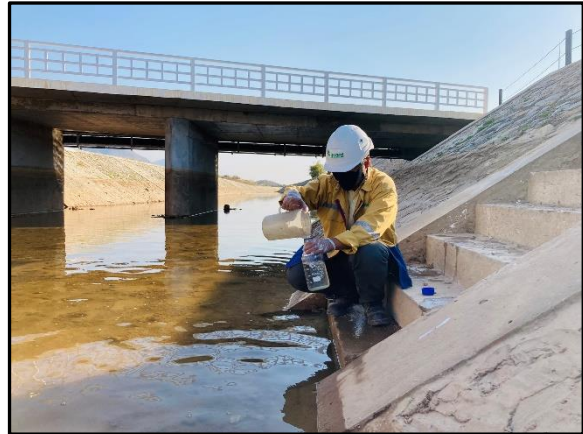
Figure 2.11: Water Quality Sampling of Surface Water
