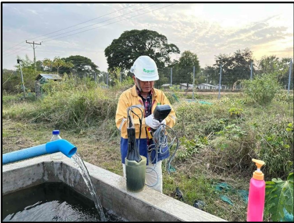
Figure 2.5.3: On-site Water Quality Measuring of Ground Water
