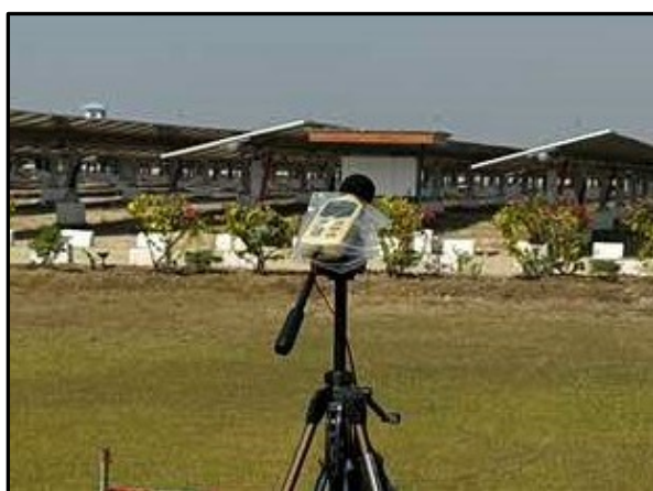
Figure 2.2.1: Noise Level Monitoring in Front of the Main Office
