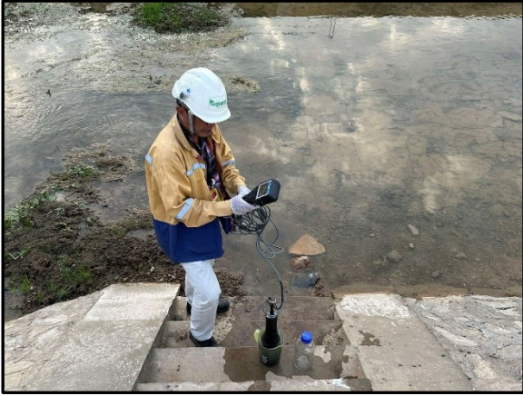
Figure 2.5.1: On-site Water Quality Measuring of Surface Water
