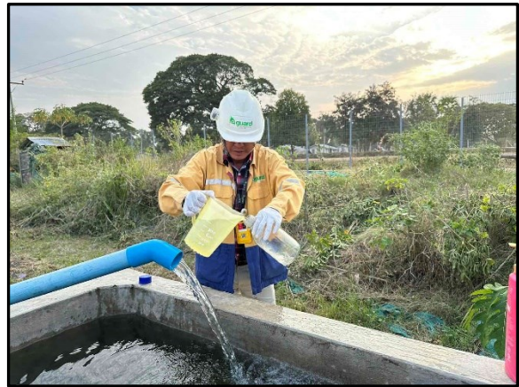
Figure 2.5.4: Water Quality Sampling of Ground Water
